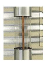
Sight Glass allows you to monitor grain flow and velocity.
